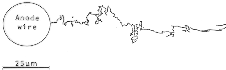
Fig. 5 Two dimensional display of a simulated drift process of one electron from starting point to anode wire surface.
