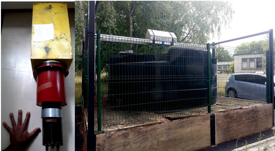
Left: Liquid organic scintillator contained in a tank (yellow). Right: Water Cherenkov detector (black).
