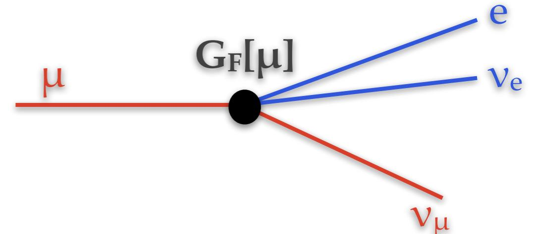
$G_F[\mu]$  measured from muon lifetime  $G_F[\mu] = 1.16637(1) \cdot 10^{-5} \text{ GeV}^{-2}$
