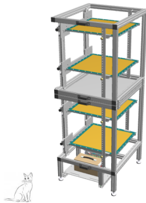
Left: tomographic bench with 4 Micromegas detectors Right: tomographic imaging of a “Muona Lisa” using lead blocks
